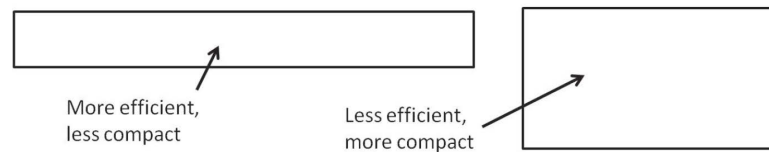
FIGURE 3.6: Wing aspect ratio trade-off: efficiency and compactness
