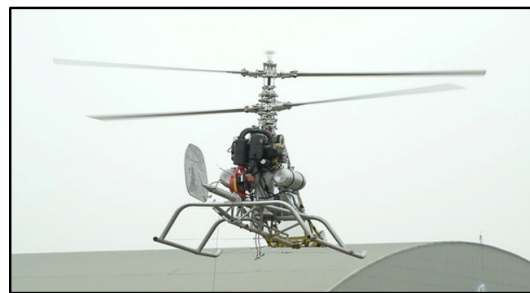
(b) Coaxial helicopter UAV
