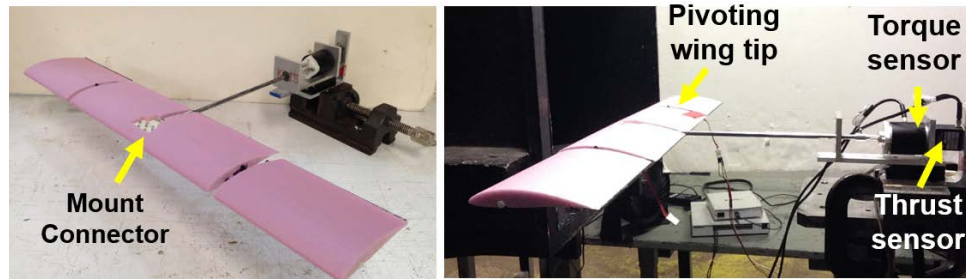
FIGURE 6.11: Wing with moving wing tip placed in front of open jet wind tunnel
