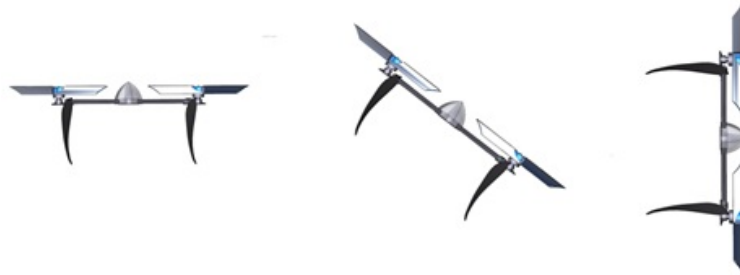
FIGURE 2.3: Equilibrium transition from hover to forward flight
